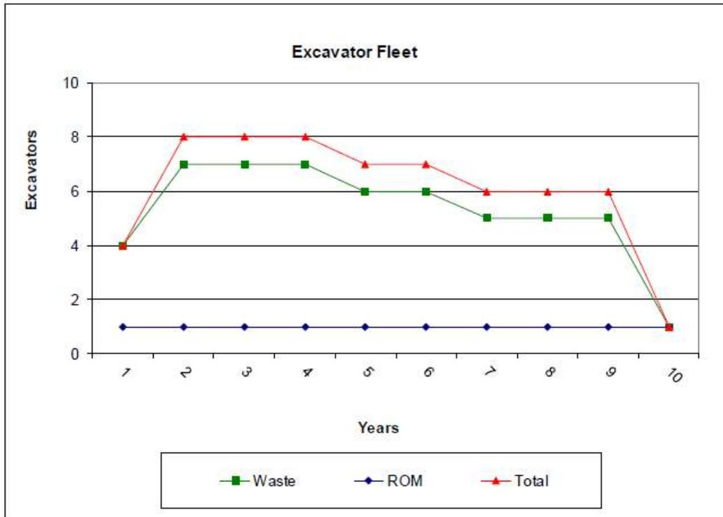
Figure 16.10 Annual excavator fleet requirements through LOM.
