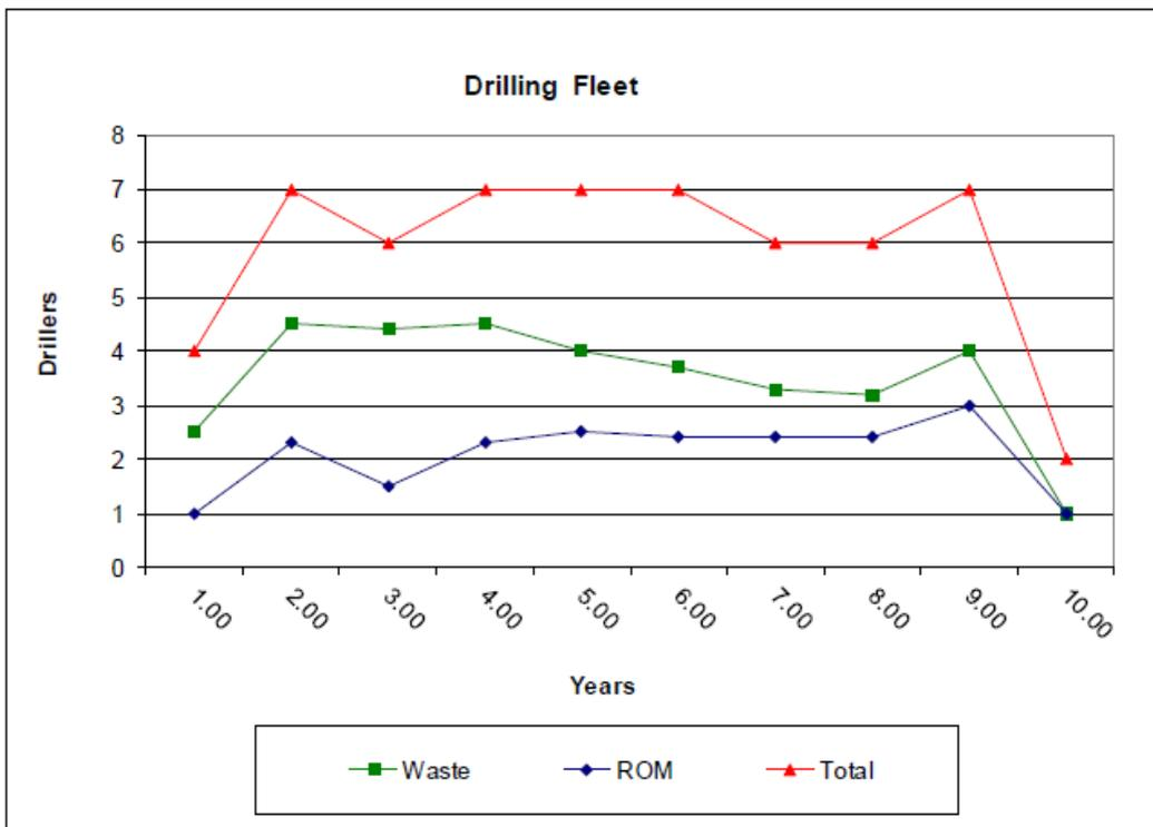
Figure 16.12 Annual Drill Rig fleet requirements through LOM.
