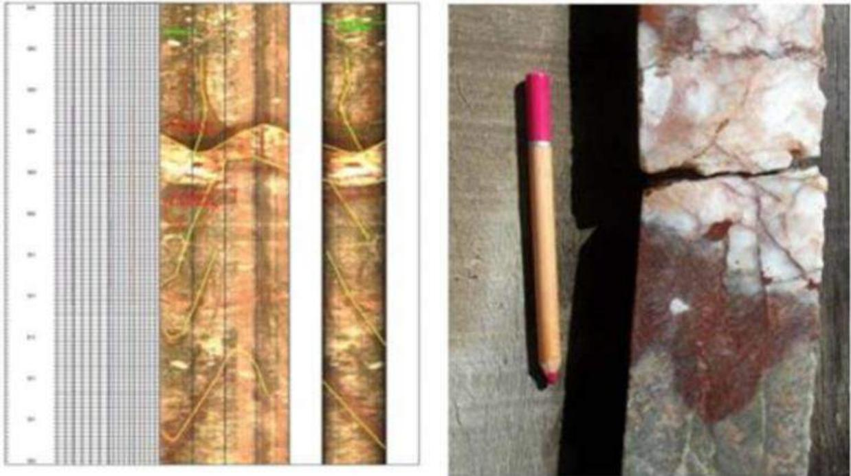
Figure 9.2 OTV image of a diamond hole compared with actual core from same interval.
