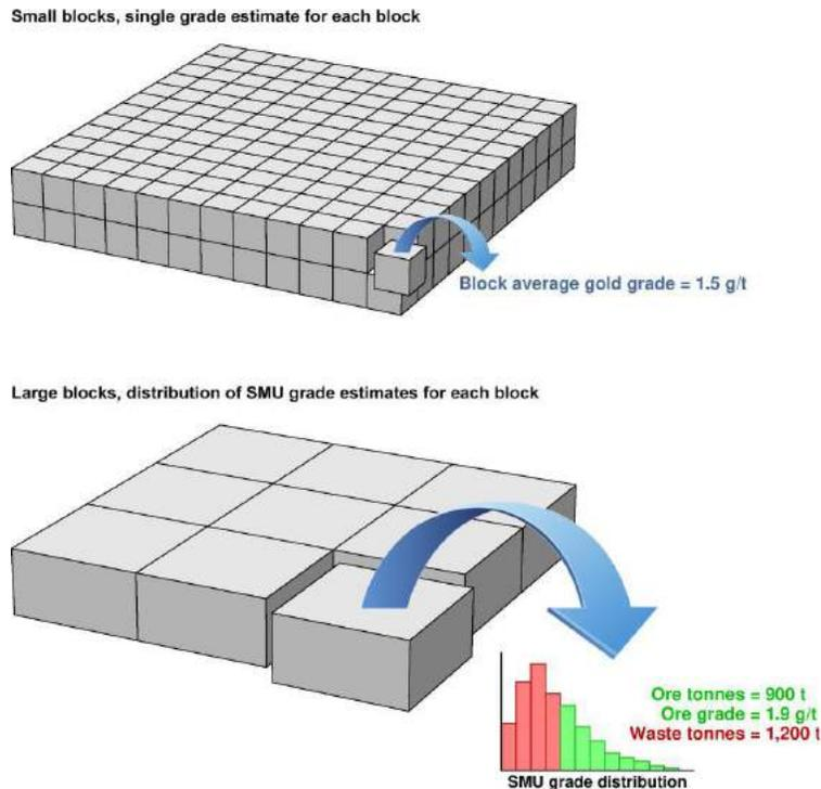
Figure 14.11 Schematic showing the difference between a conventional single-estimate block model and a recoverable-resources block model that provides an estimate of the SMU grade distributions within large blocks.
