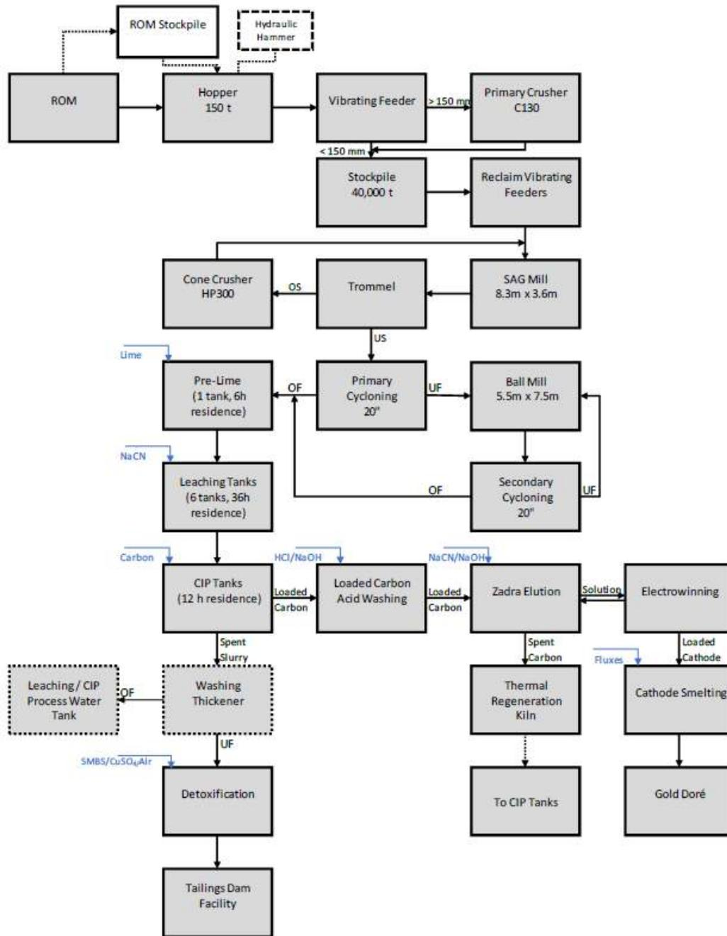
Figure 17.1 Simplified Block Diagram Proposed Flowsheet.
