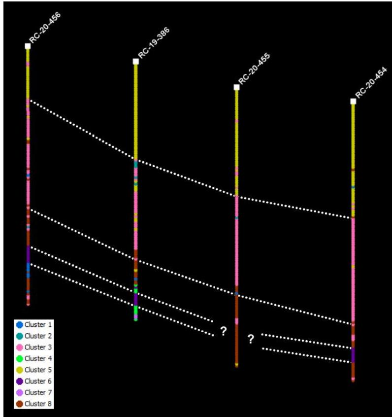
Figure 9.4 Example of clusters developed by machine learning from 4A-ICP multi-element chemistry, and correlatable from hole to hole, with interpretation of marker horizons.
