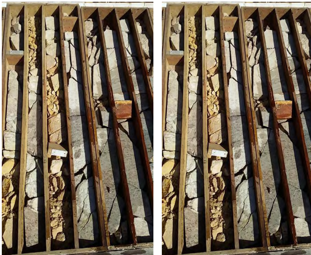
Figure 16-5: Drillcore box in transition from saprolitic to fresh-rock zone with local friable intercepts (shallow than 43m depth)
